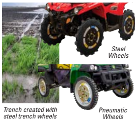
Trench created with steel trench wheels
